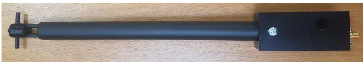
Figure 1 – MVG COMOSAR Validation Dipole
