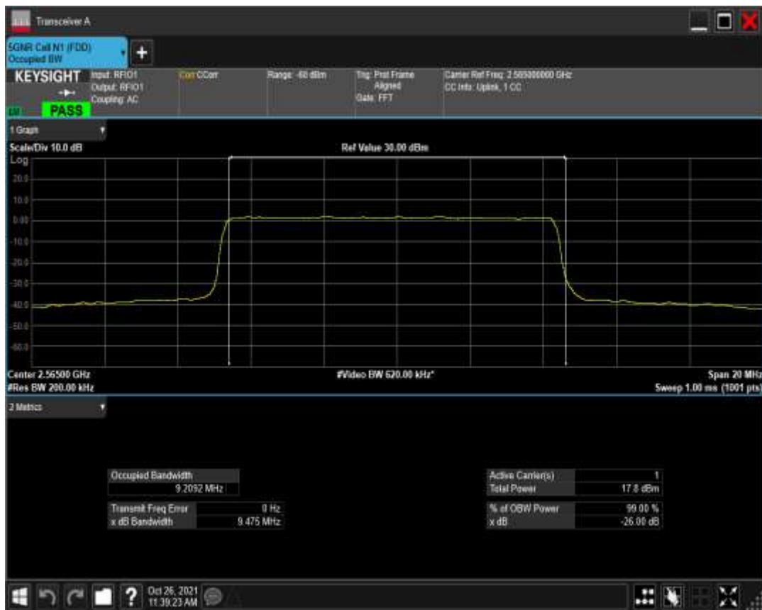
n7 SCS=15kHz DFT_QAM256 BW=15MHz Channel=501500 RB=75@0
