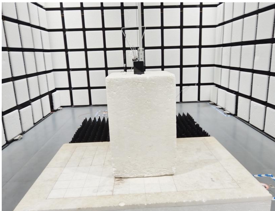
Radiated spurious emission Test Setup-2(Above 1GHz)
