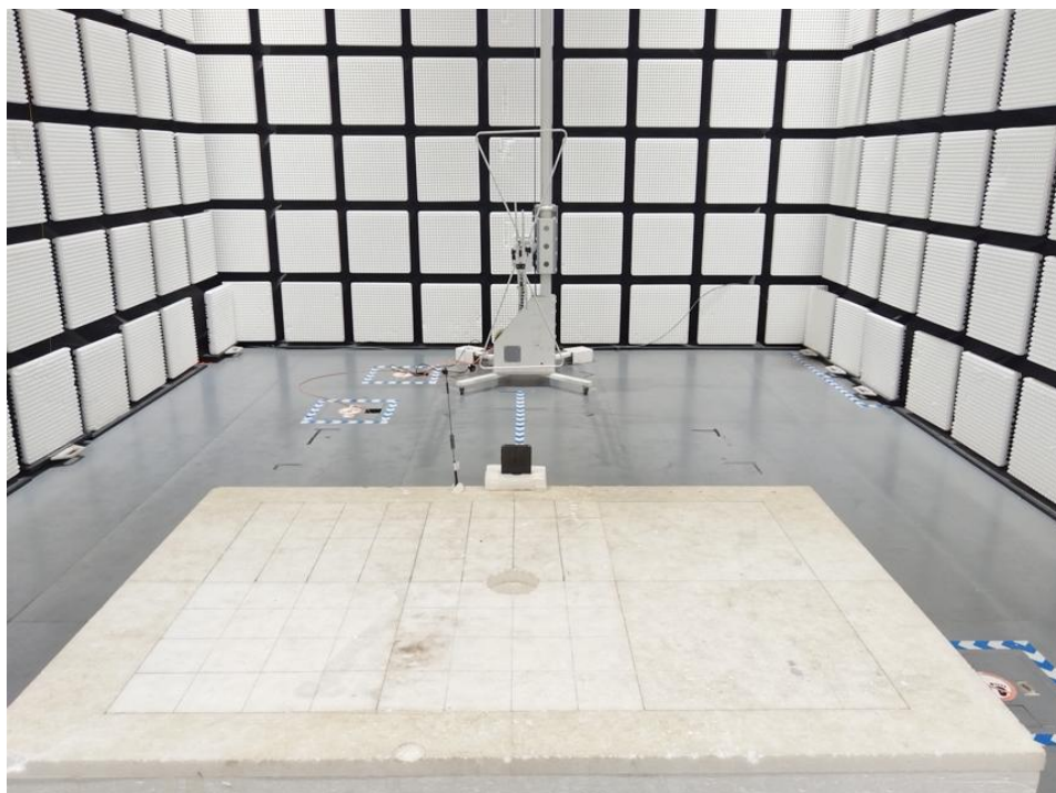
Radiated spurious emission Test Setup-2(Above 1GHz)
