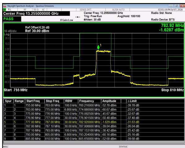
n13 SCS=15kHz DFT_16QAM BW=5MHz HighChannel=156900 RB=25@0
