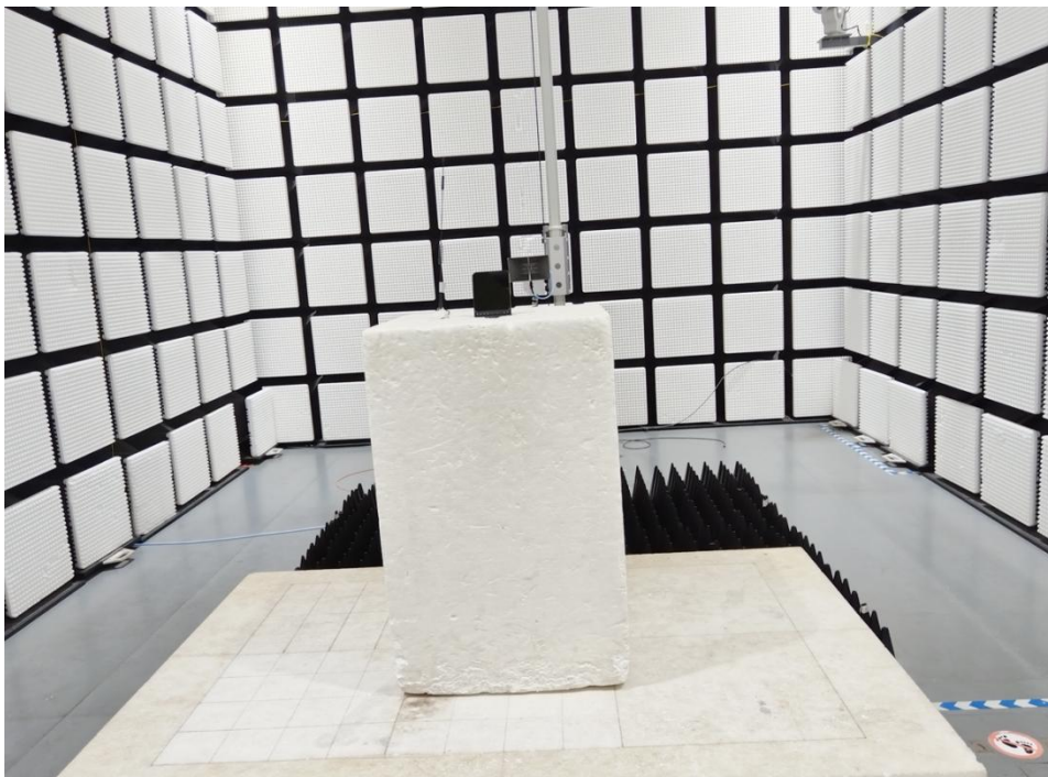
Radiated spurious emission Test Setup-2(Above 1GHz)
