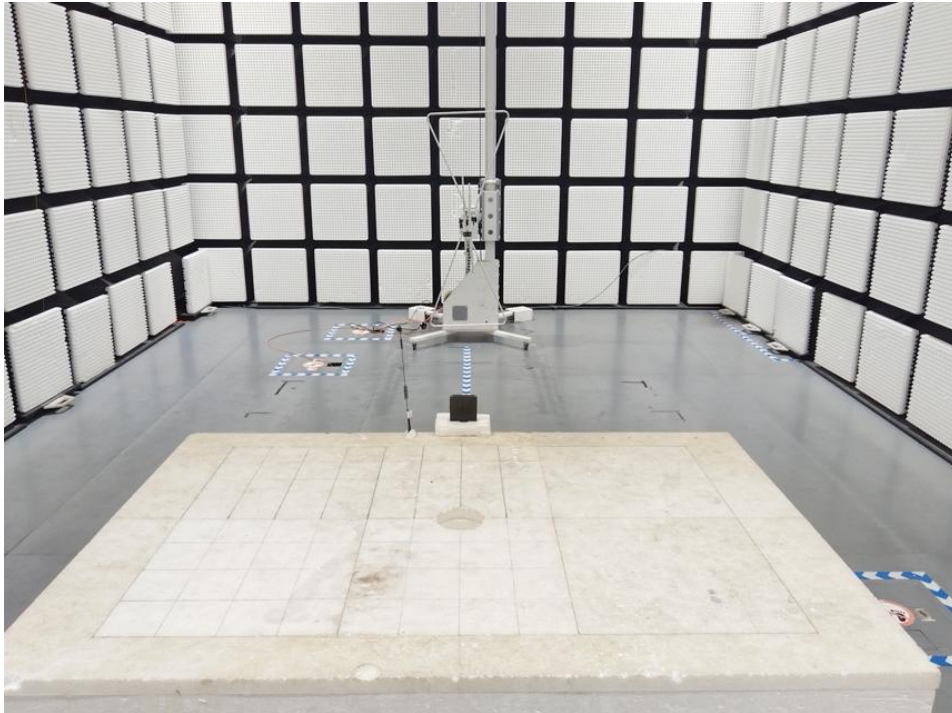
Radiated spurious emission Test Setup-2(Above 1GHz)
