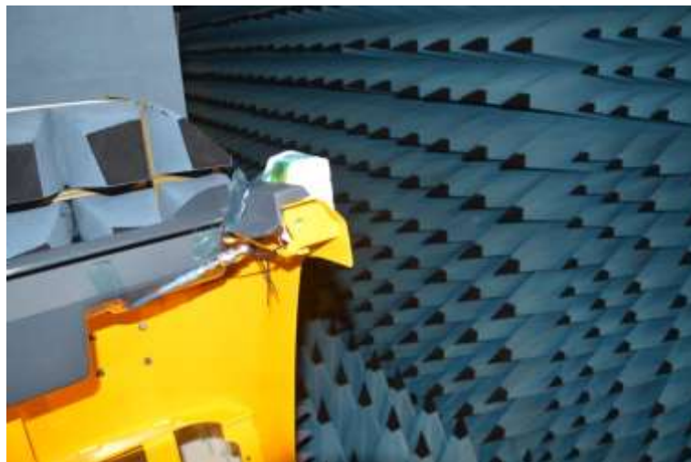
Figure 3-37 UWB Antenna with vehicle parts in position A (front)
