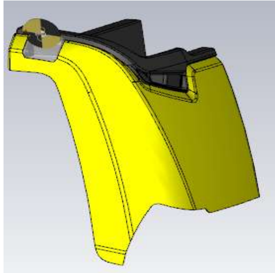
Figure 24: Simulation model for the front right antenna including the nearby elements of the vehicle.
