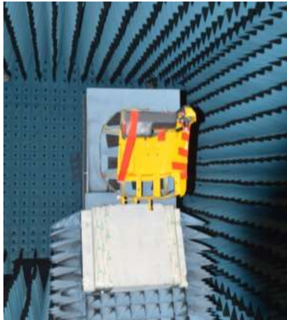
Figure 65: Front side nearby vehicle components and the antenna positioned for the measurement.
