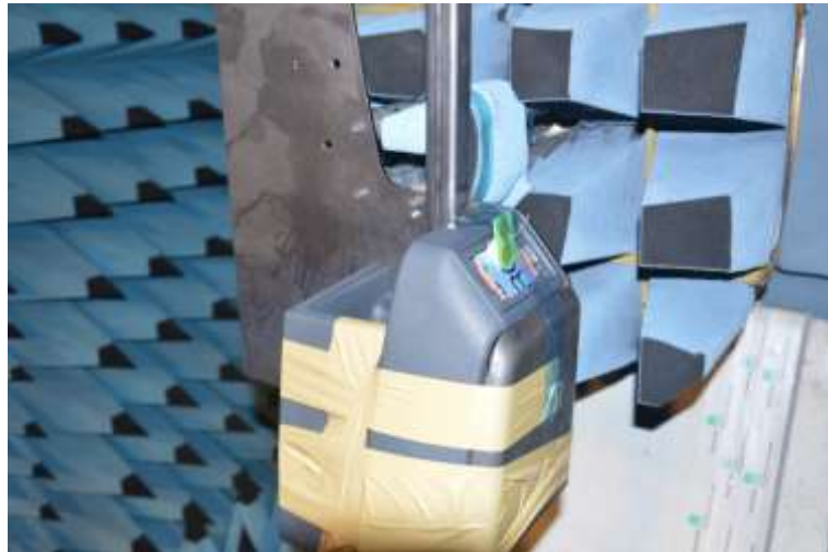
Figure 3-36 UWB Antenna with vehicle parts in position B (back)
