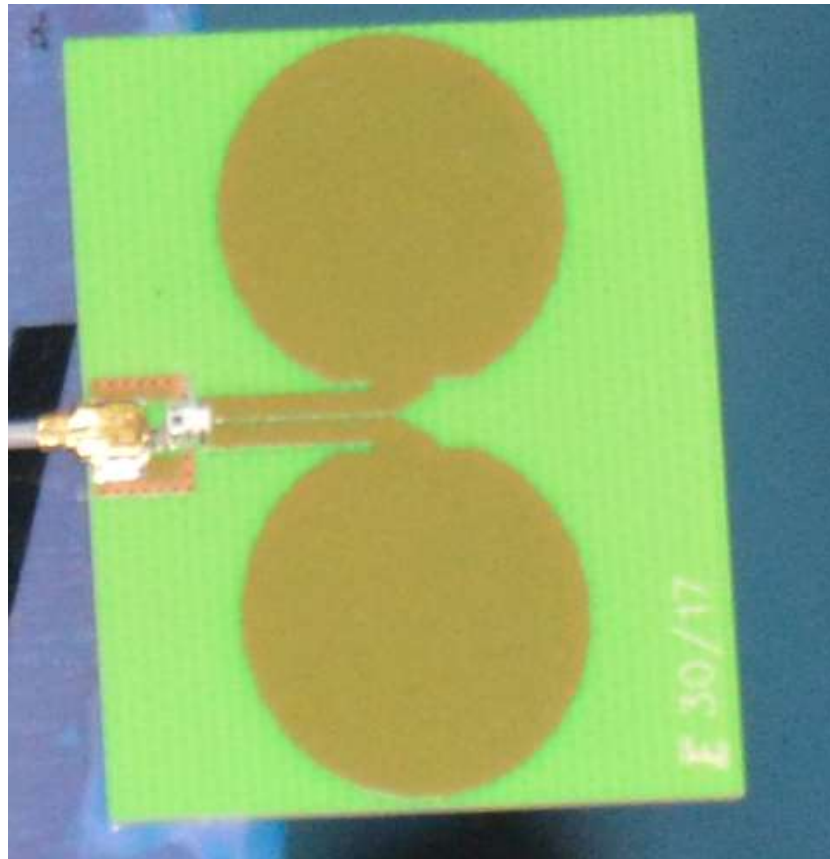
Figure 4: The antenna with chip balun circuitry
