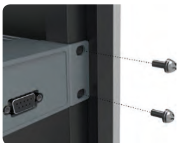
Fig. 11: Fix C-hub with screws
