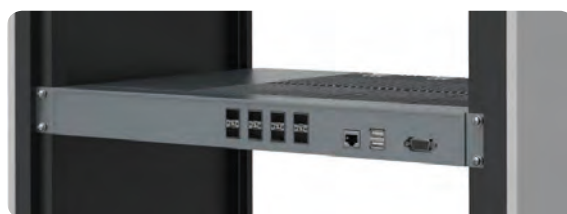
Fig. 10: Place C-hub in rack
