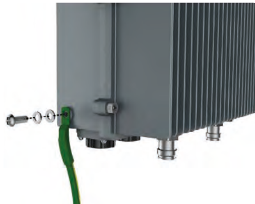
Fig. 29: Connect ground cable at bottom side
