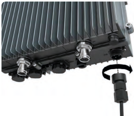
Fig. 28: Connect power cable at bottom side
