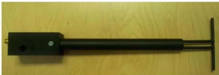
Figure 1 – MVG COMOSAR Validation Dipole
