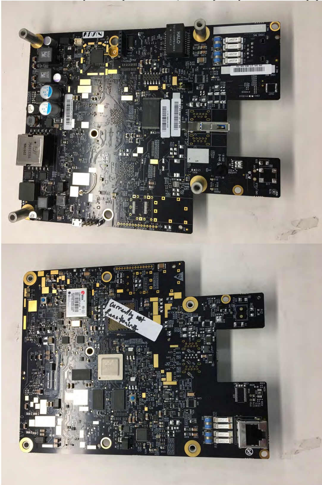
Main PCB- Secondary board top and bottom (Same as primary main board - depopulated)
