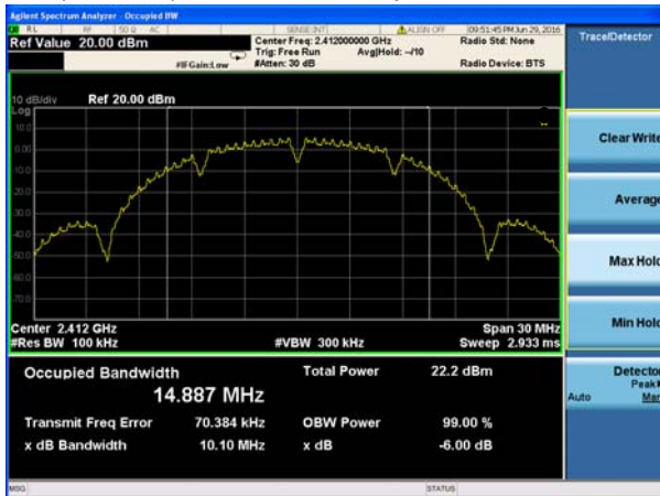
(802.11b) 6dB Bandwidth plot on channel 1
