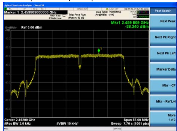
(802.11n40) PSD plot on channel 9
