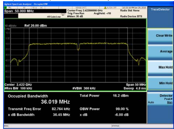
(802.11n40) 6dB Bandwidth plot on channel 3
