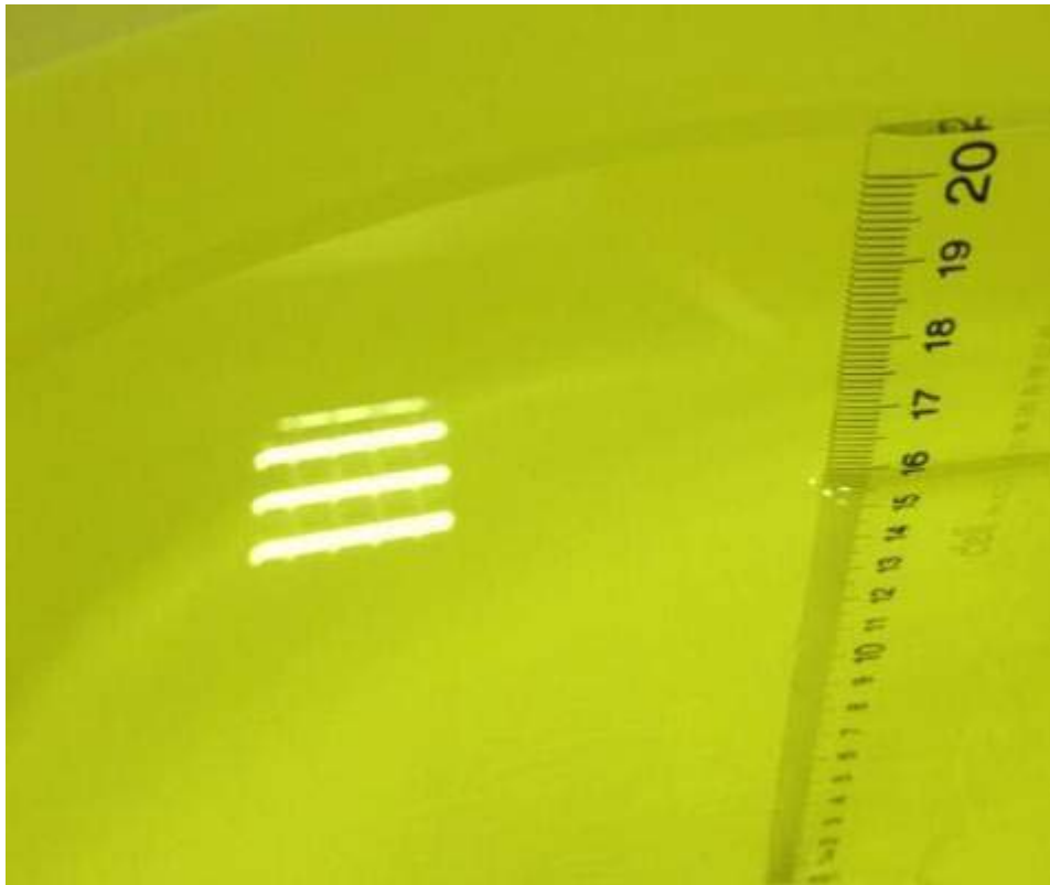
Picture 8-3: Liquid depth in the Head Phantom (2450 MHz Head)
