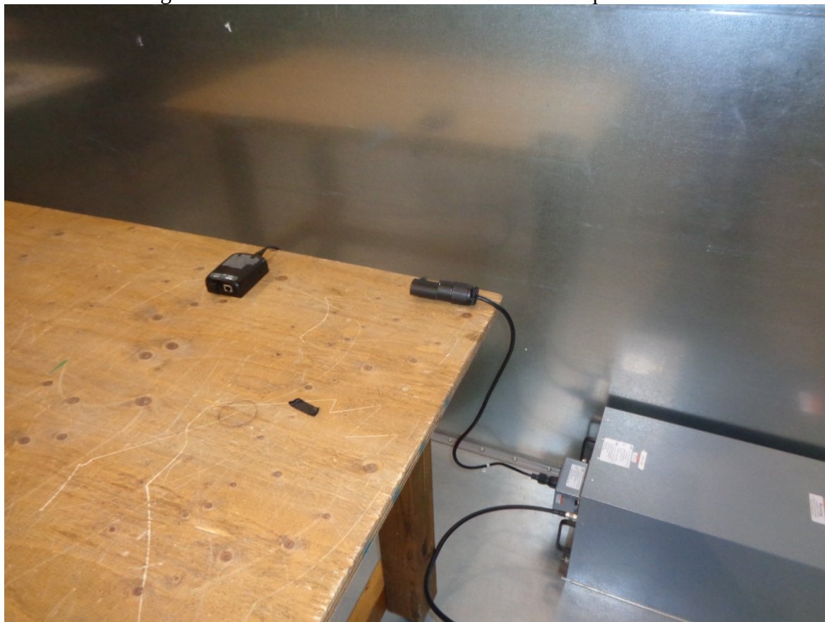
Figure 5 – Power Line Conducted Emissions Setup – Photo 2
