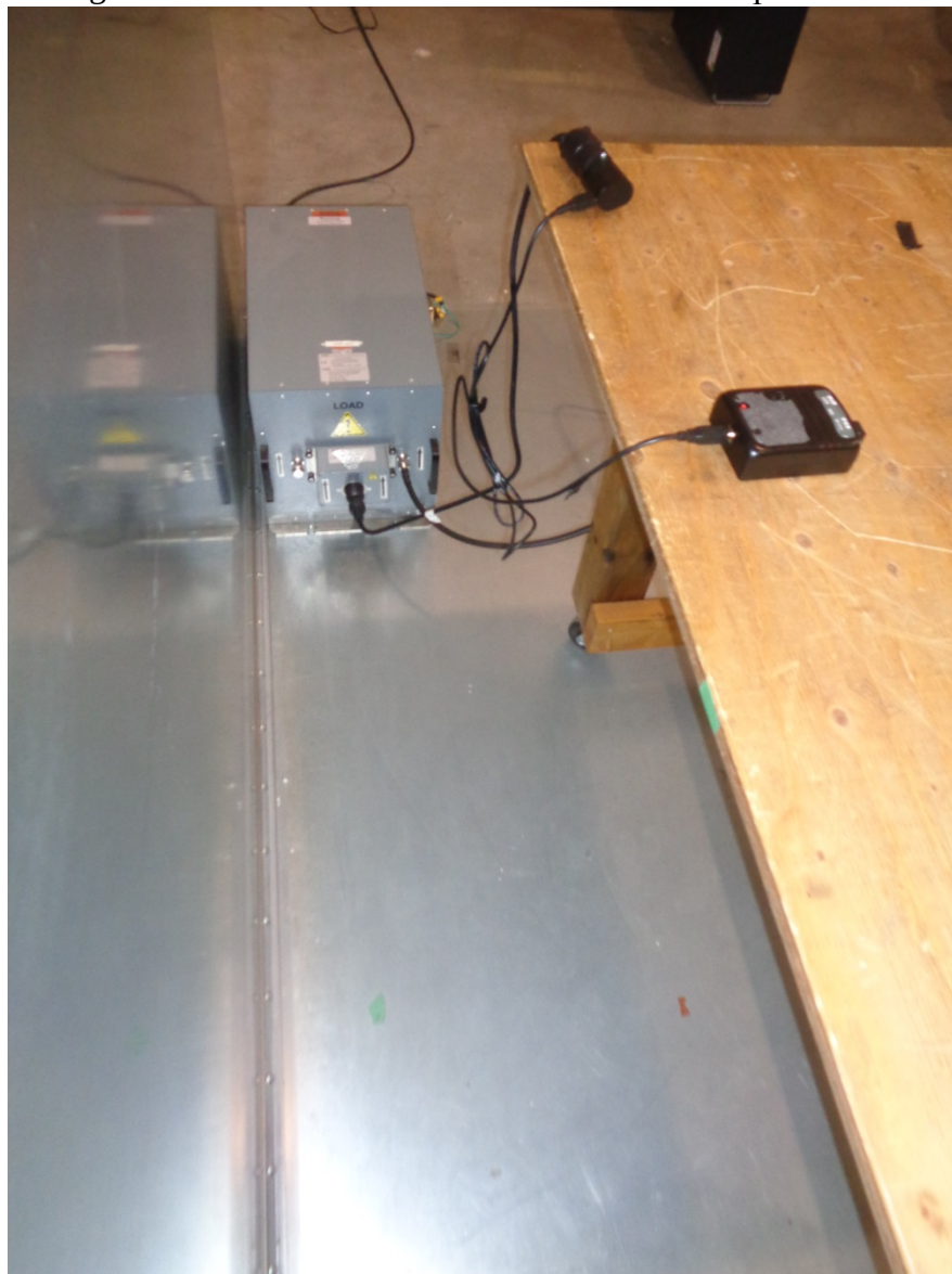
Figure 4 – Power Line Conducted Emissions Setup – Photo 1
