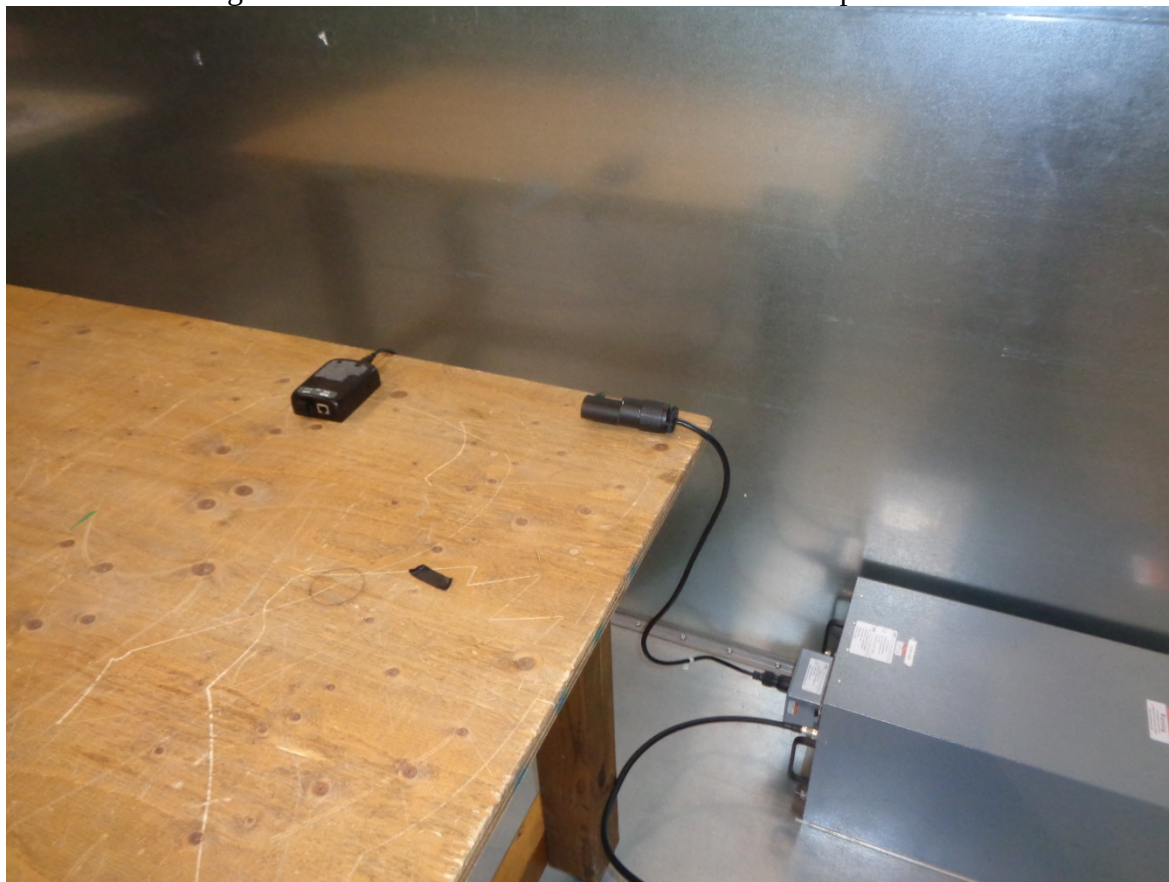
Figure 5 – Power Line Conducted Emissions Setup – Photo 2
