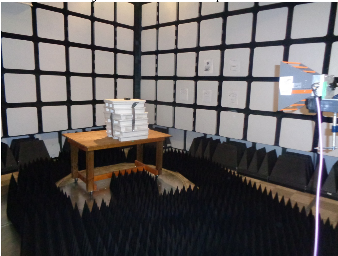
Figure 3 – Radiated Emissions Setup – Photo 3
