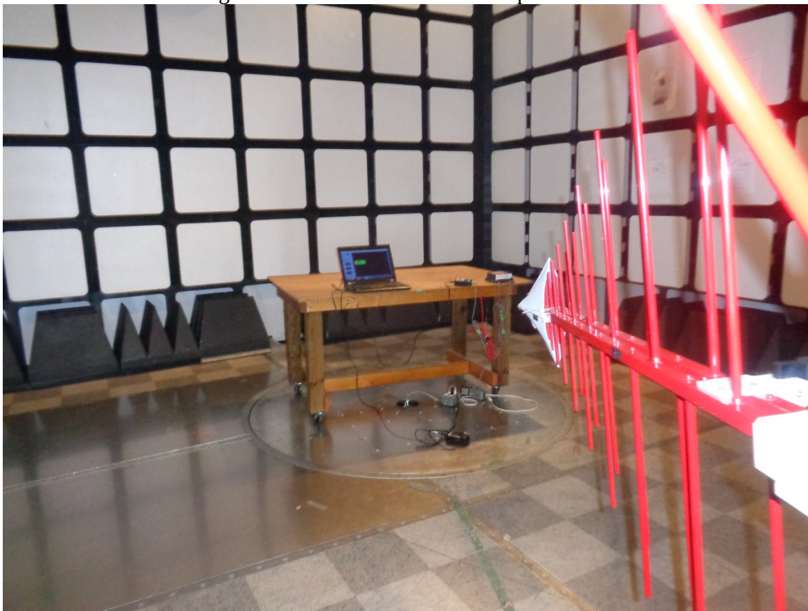
Figure 1 – Radiated Emissions Setup – Photo 1
