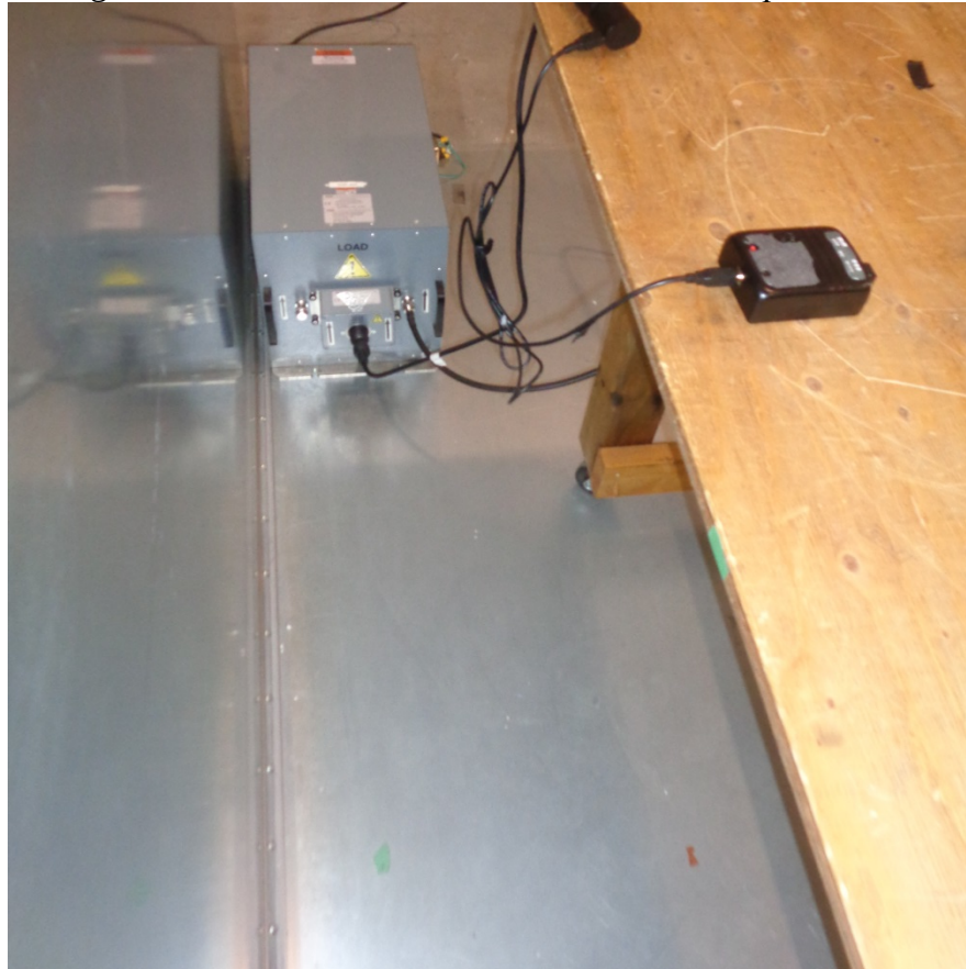
Figure 4 – Power Line Conducted Emissions Setup – Photo 1
