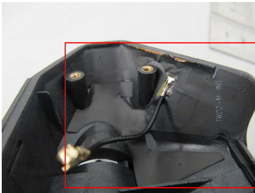
EUT – WCDMA & LTE Main Antenna View
