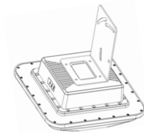
Picture 0-1 wall installation
