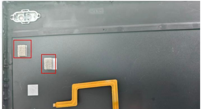
Conductive sponge is attached to the laser-engraved position on the back shell to connect the shield
