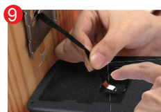
Connect cable socket to connection base.
