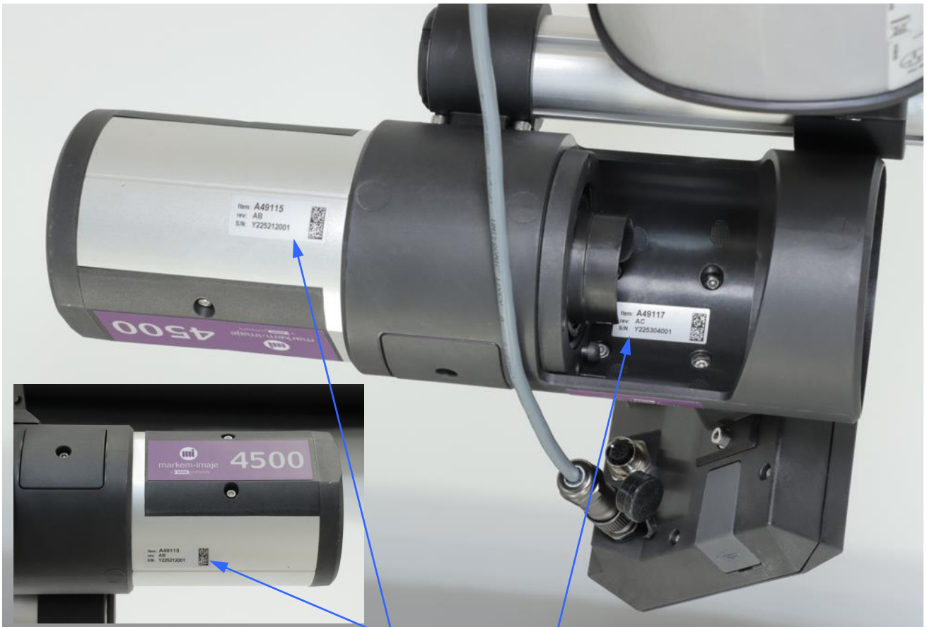
Fig. 4. Printhead module identification label
