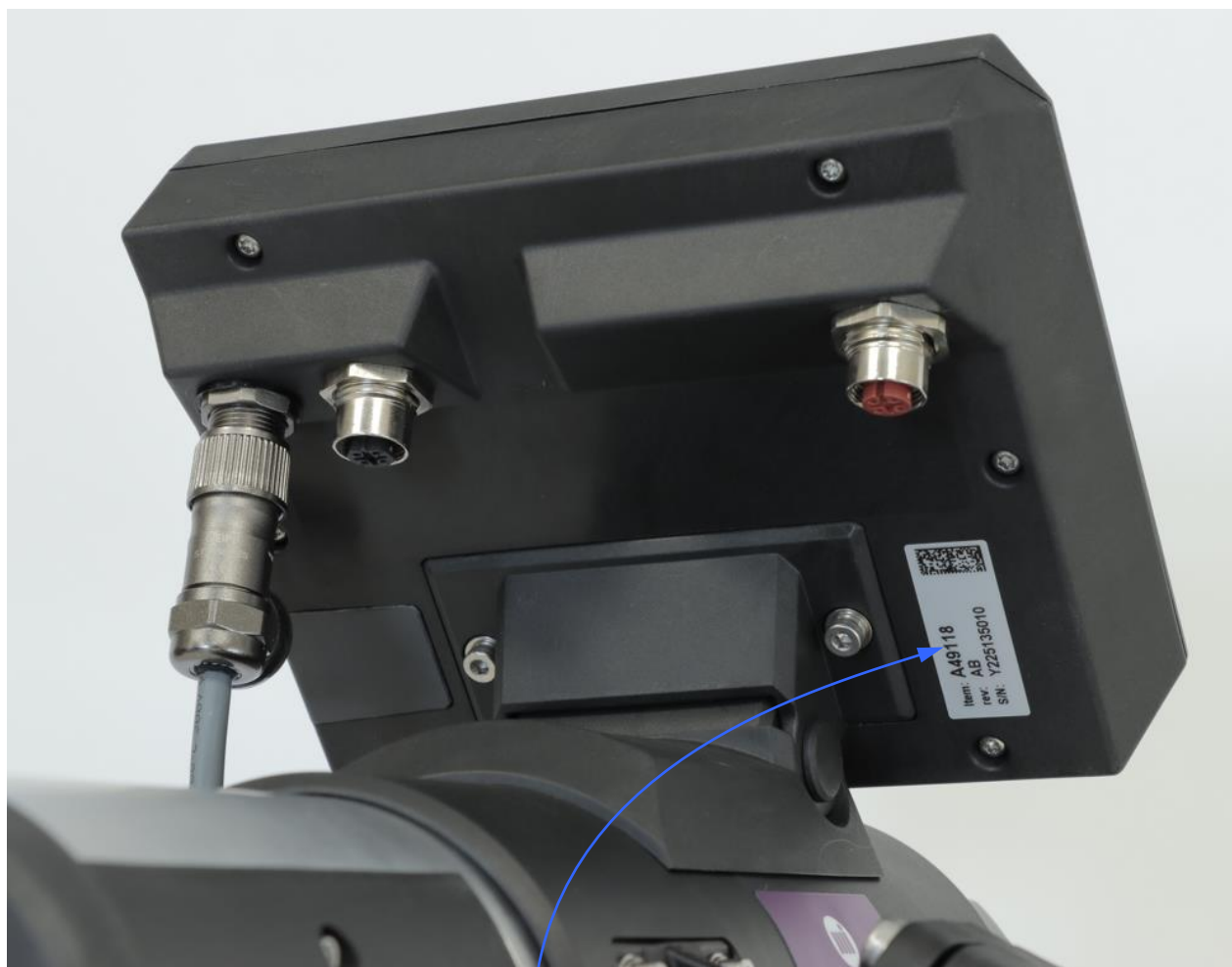
Fig. 3. Control Unit module identification label
