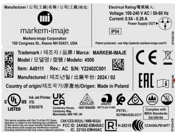
Example name plate of complete 4500 printer, variant A49111, located on the side of the A49119 Power Supply module
