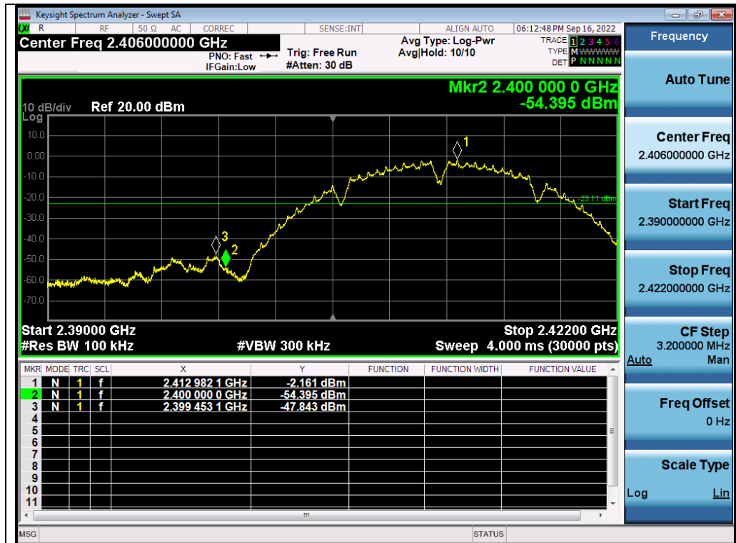
Test_Graph_802.11b_ANT1_2412_1Mbps_Lower Band Edge Emissions
