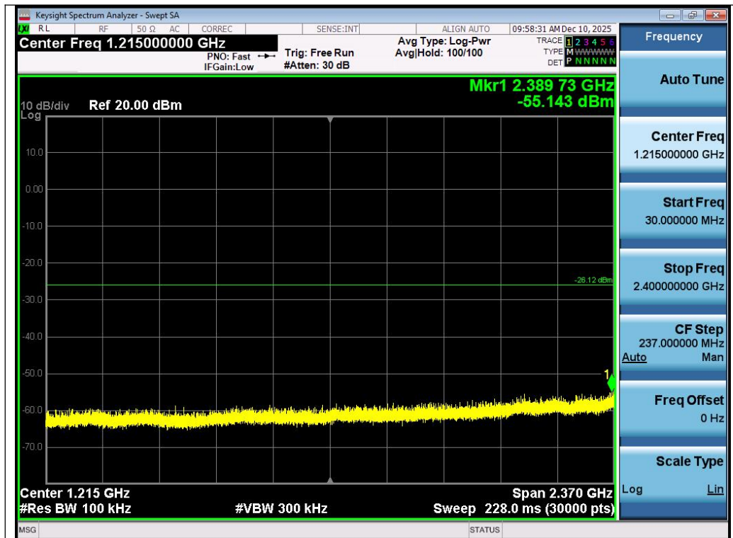
Test_Graph_802.11n40_ANT1_2452_MCS0_Lower Band Emissions
