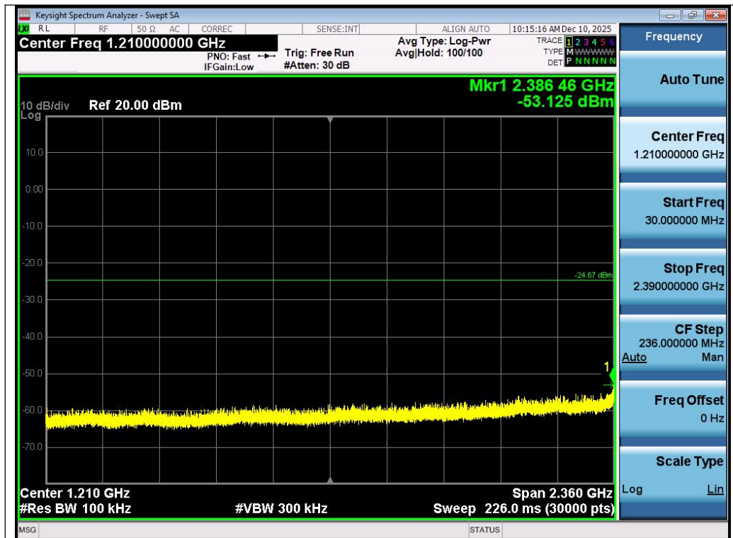
Test_Graph_802.11ax40_ANT1_2422_MCS0_Lower Band Emissions
