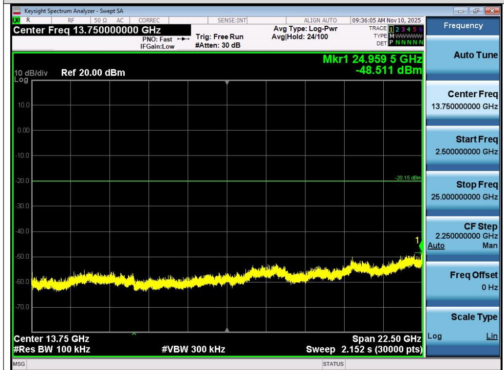
Test_Graph_802.11ax20_ANT1_2462_MCS0_Higher Band Emissions
