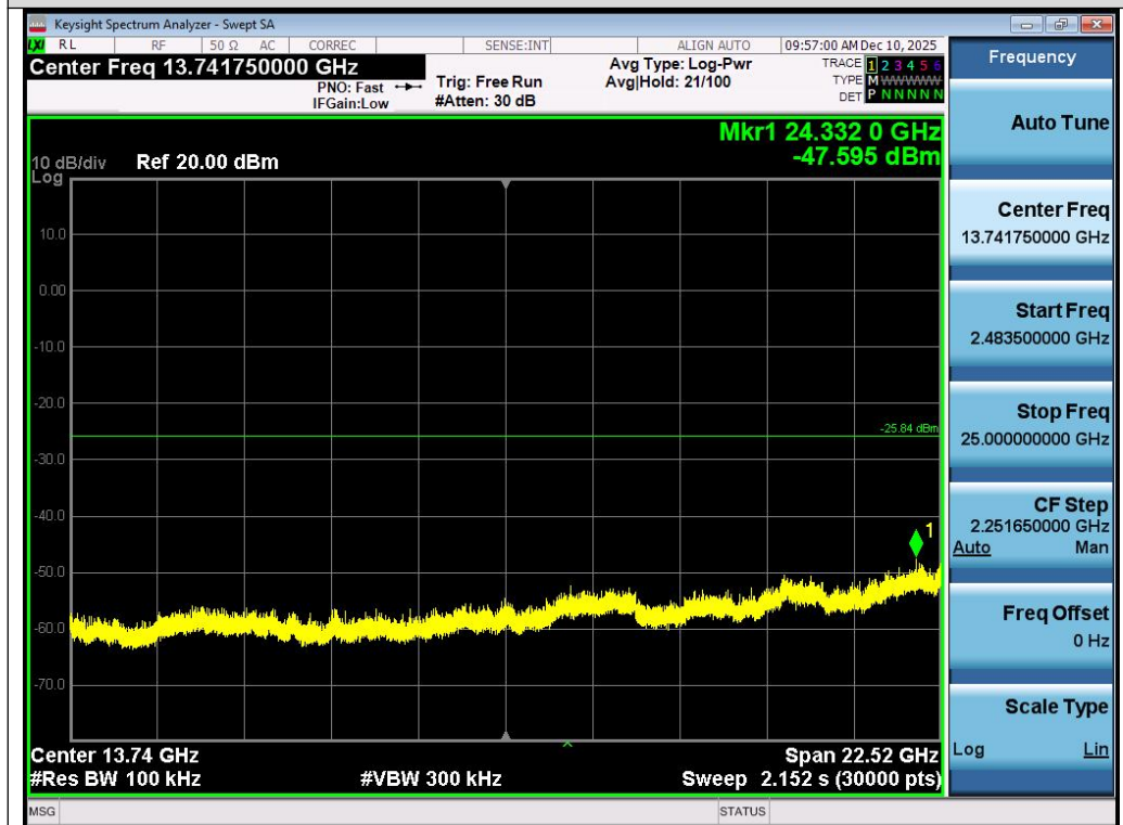
Test_Graph_802.11n40_ANT1_2437_MCS0_Higher Band Emissions
