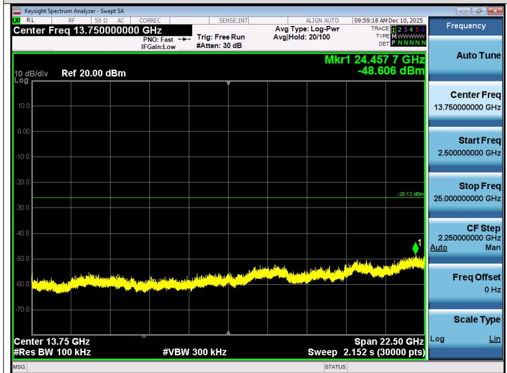
Test_Graph_802.11n40_ANT1_2452_MCS0_Higher Band Emissions
