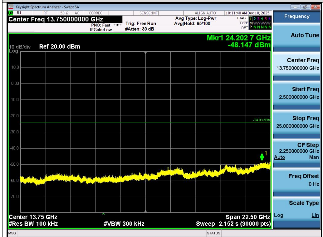
Test_Graph_802.11ax20_ANT1_2437_MCS0_Higher Band Emissions
