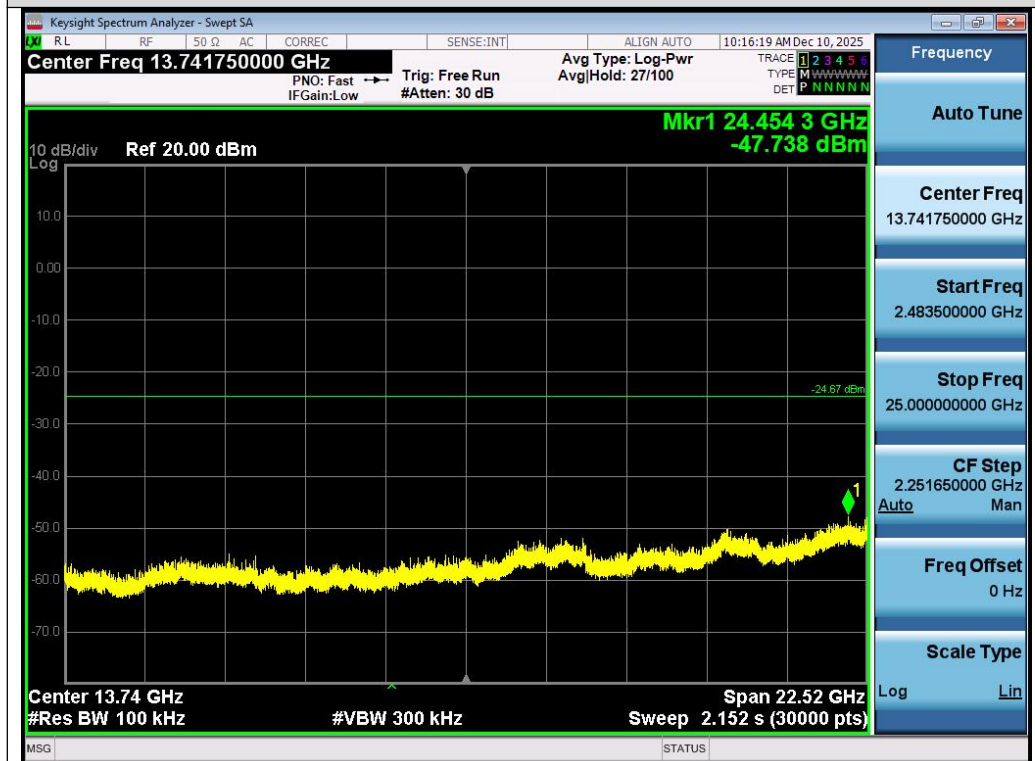
Test_Graph_802.11ax40_ANT1_2422_MCS0_Higher Band Emissions
