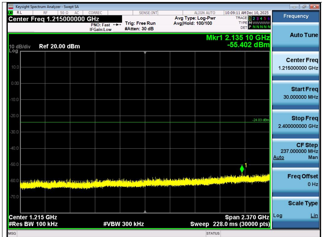
Test_Graph_802.11ax20_ANT1_2437_MCS0_Lower Band Emissions
