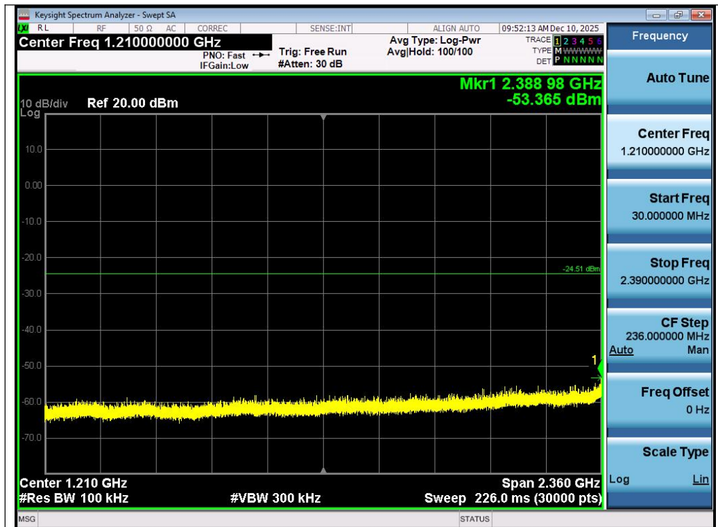
Test_Graph_802.11n40_ANT1_2422_MCS0_Lower Band Emissions
