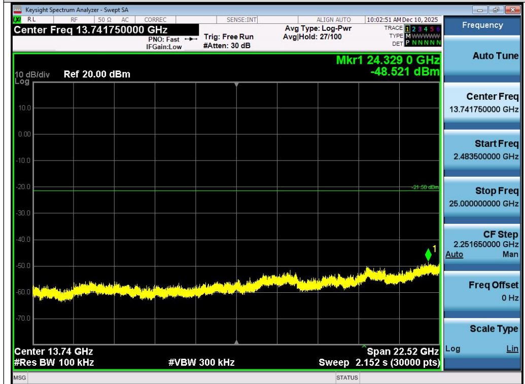
Test_Graph_802.11ax20_ANT1_2412_MCS0_Higher Band Emissions
