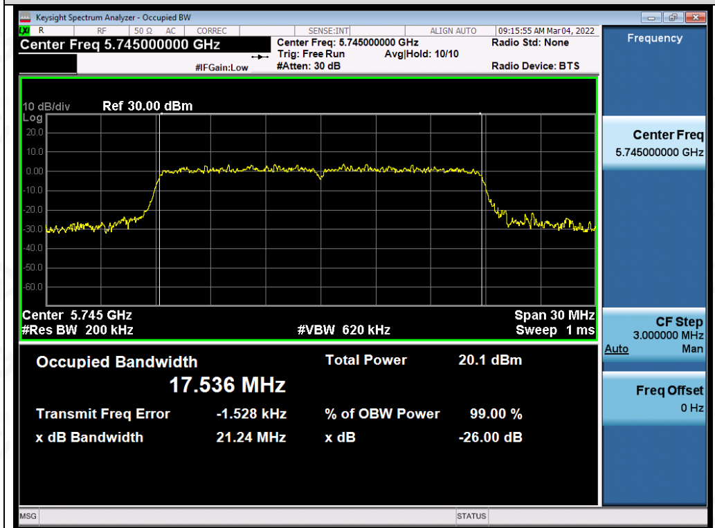
Test_Graph_802.11n20_ANT1_5745_MCS0_OBW
