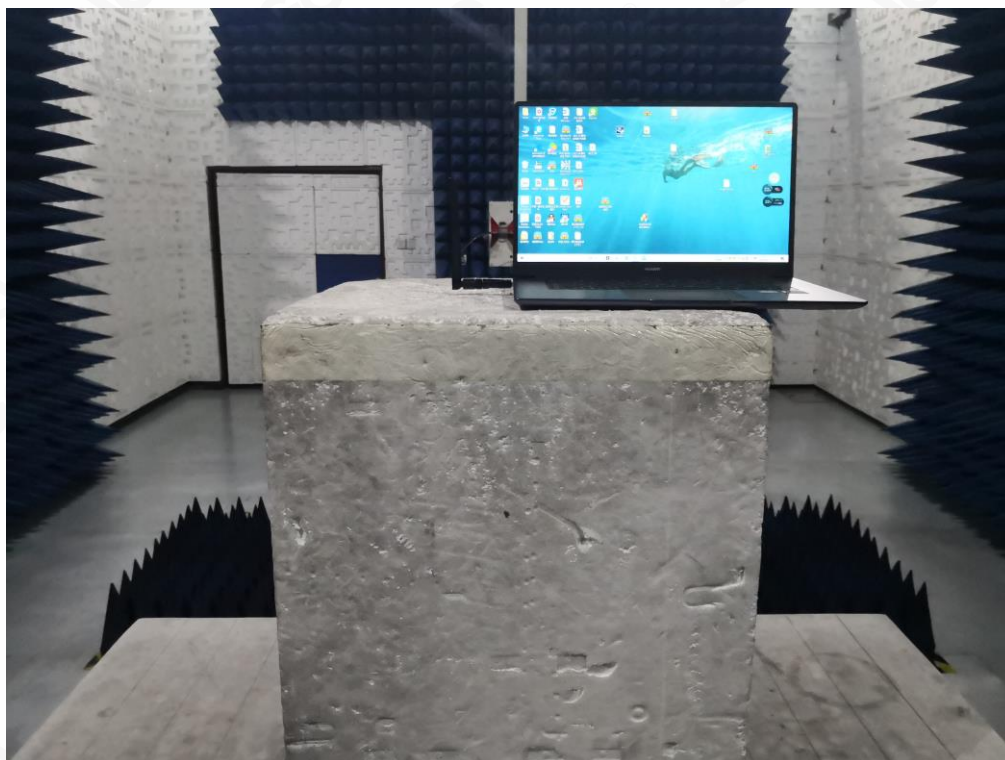
FCC RADIATED EMISSION TEST SETUP ABOVE 1GHZ
