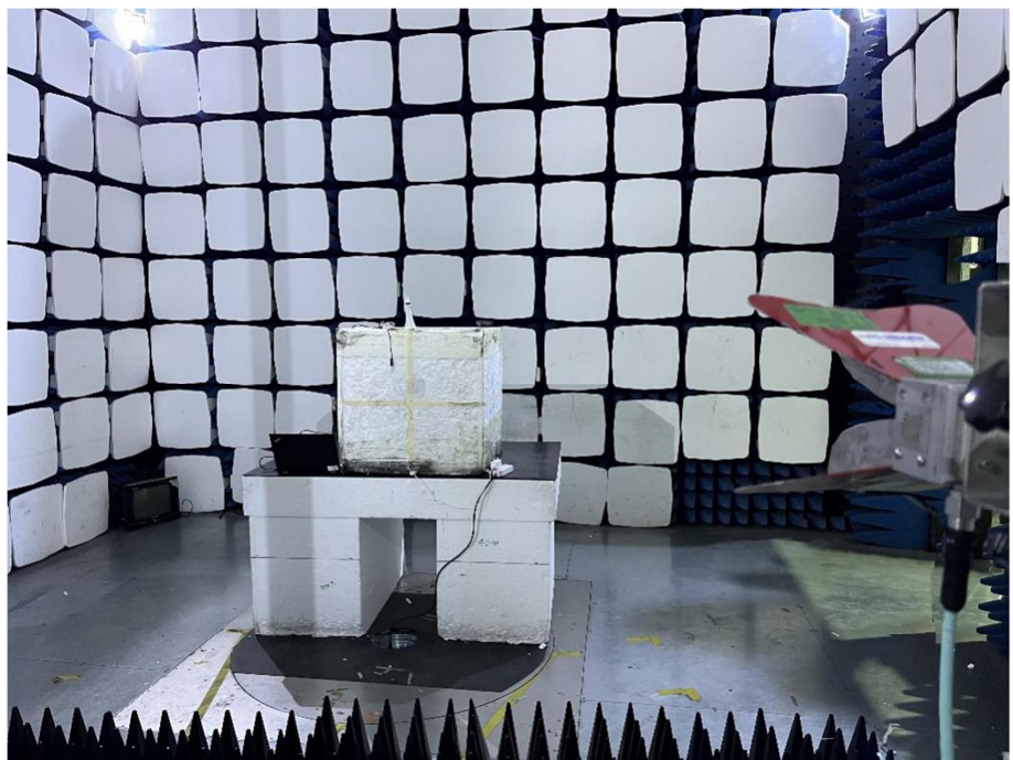
Radiation Emission Test Setup (1GHz to 18GHz)
