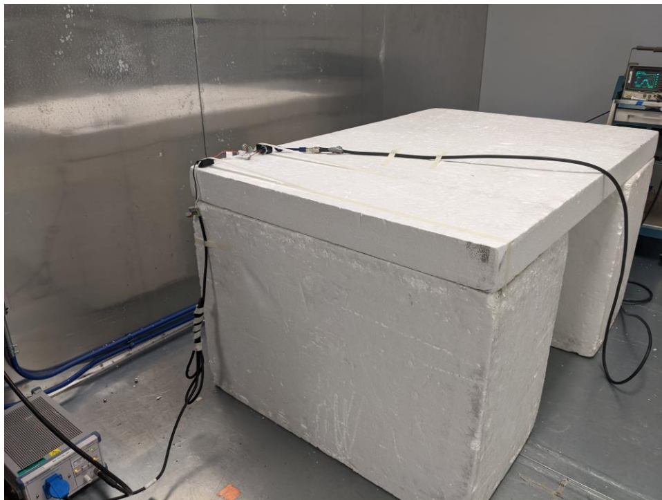
Figure 7: Test Setup – Conducted Emissions
