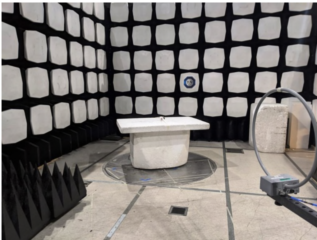
Figure 2: Equipment Under Test – Radiated Emissions <30MHz
