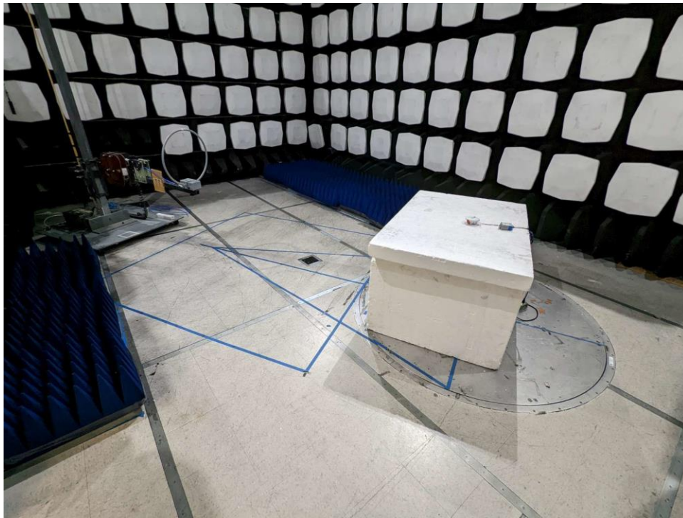
Figure 1: Test Setup – Radiated Emissions <30MHz
