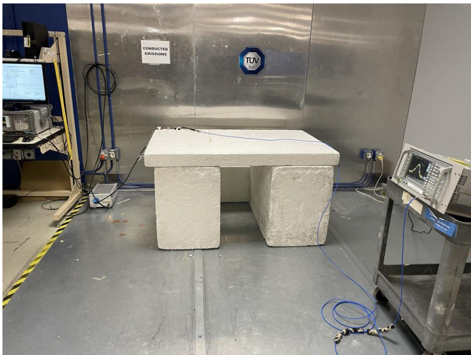
Figure:12– Front view of Test Set up – Power Line Conducted Emissions
