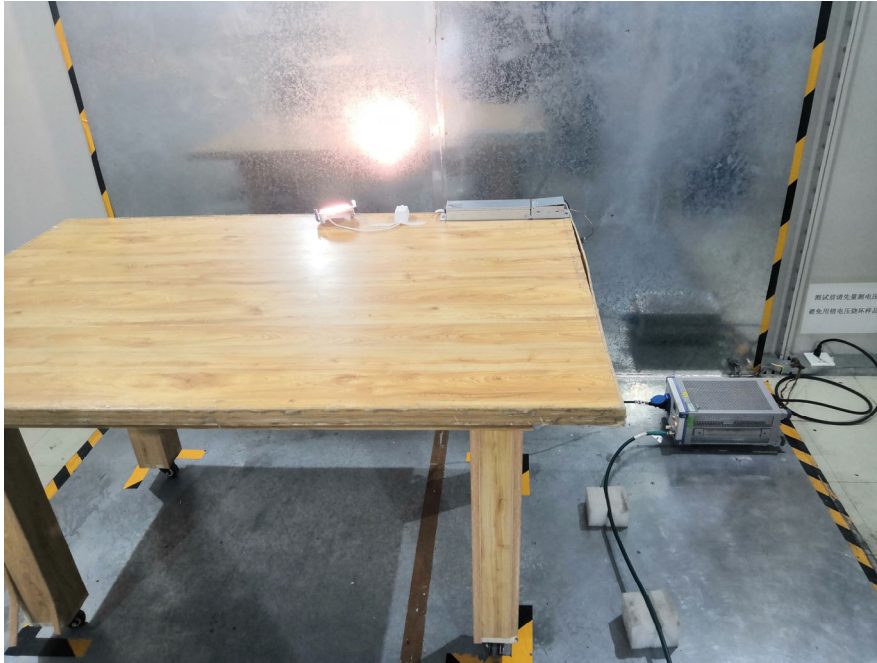
Conducted Emissions (Side View)
