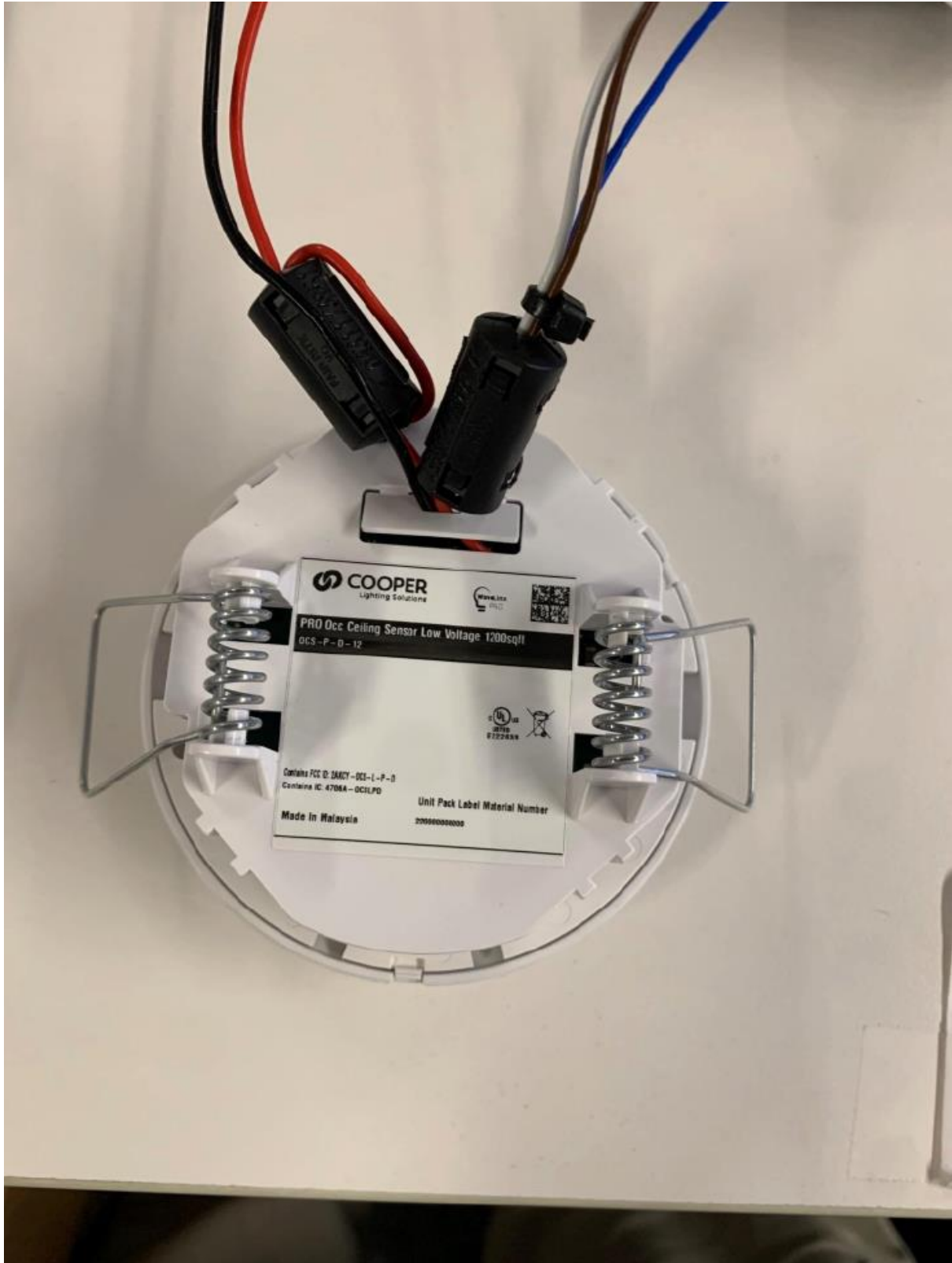
Label Location – Low Voltage
