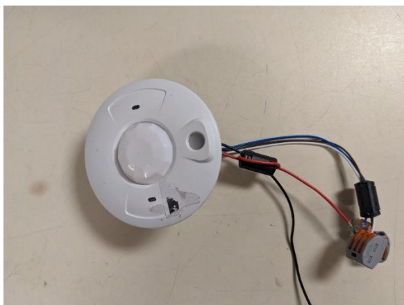
Photo 1.4.1-1 – Front view of the DC EUT
