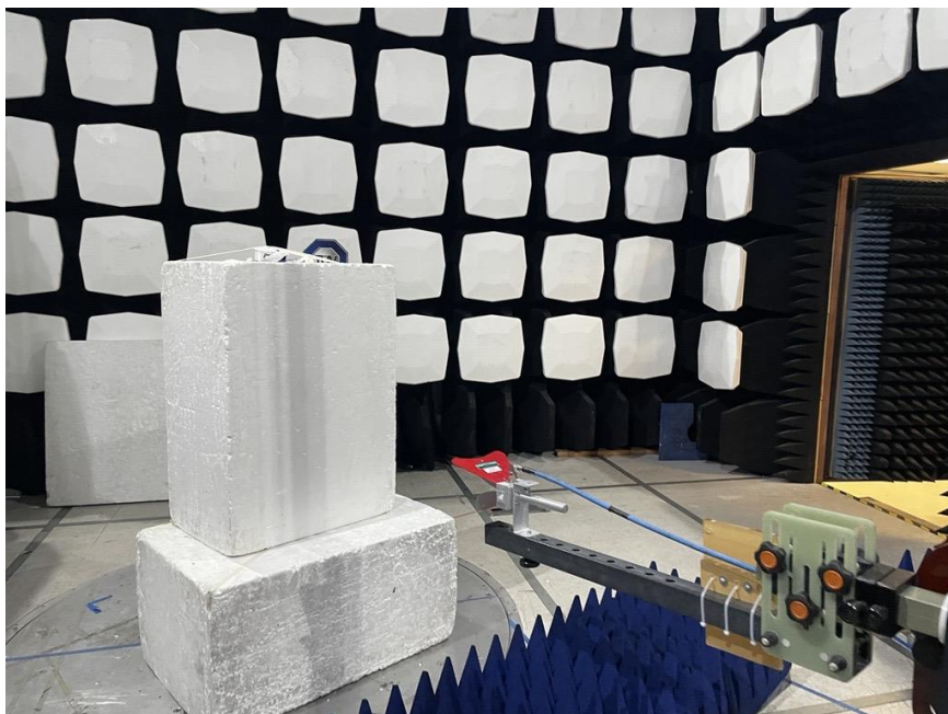
Figure:7– Test Set up – Front View of the EUT - Radiated Emissions <18 GHz
