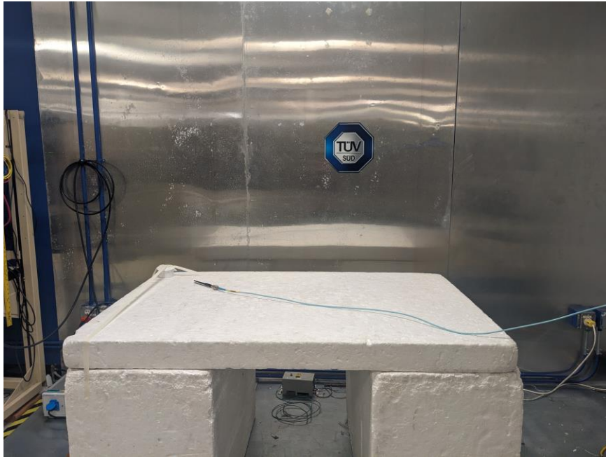
Figure:9– Test Set up – Power Line Conducted Emissions
