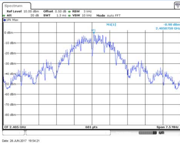
O-QPSK LOW CHANNEL
