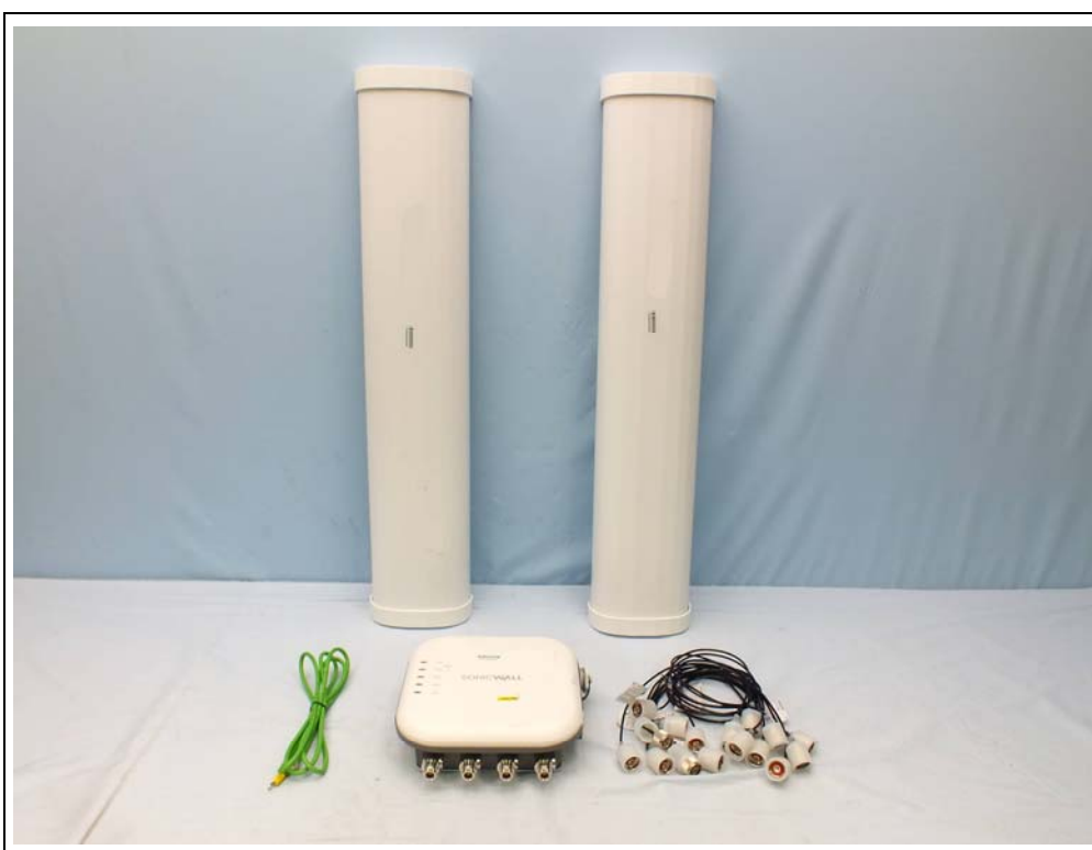
EUT with Sector antenna
