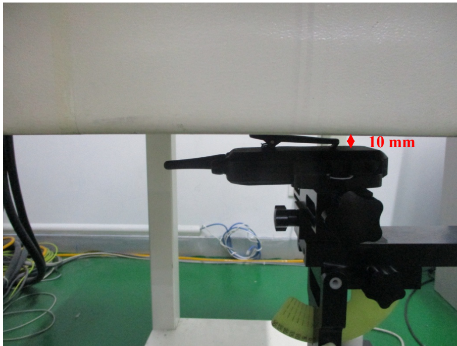
Body Back Setup Photo(10mm)
