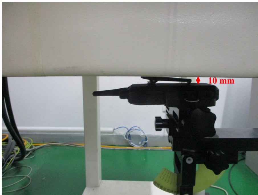
Body Back Setup Photo(10mm)
