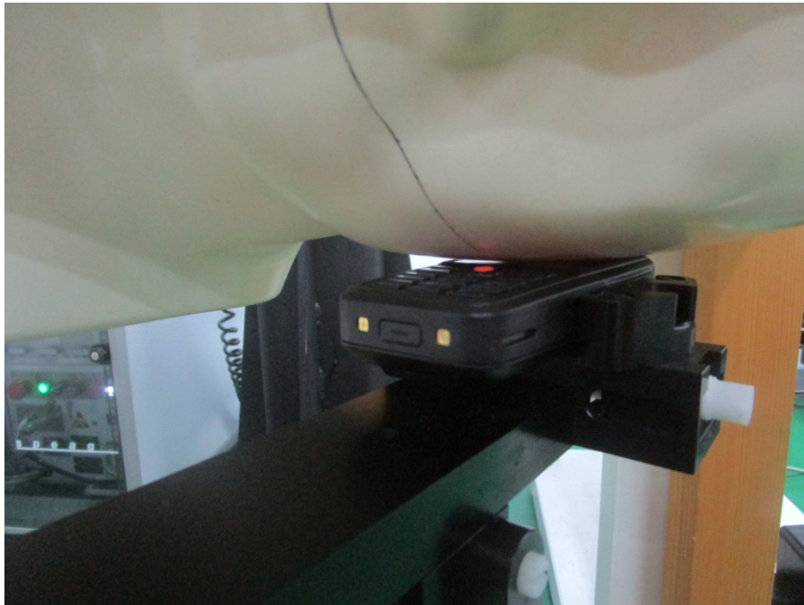
Head Left Cheek Setup Photo
