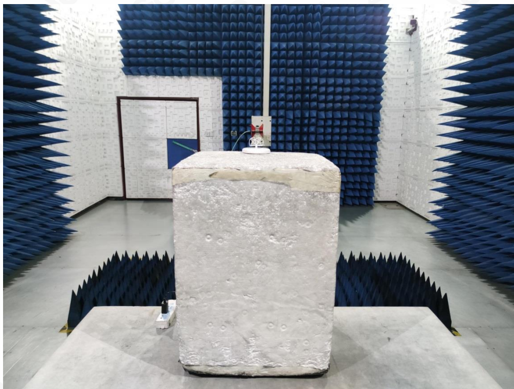
FCC RADIATED EMISSION TEST SETUP ABOVE 1GHZ
