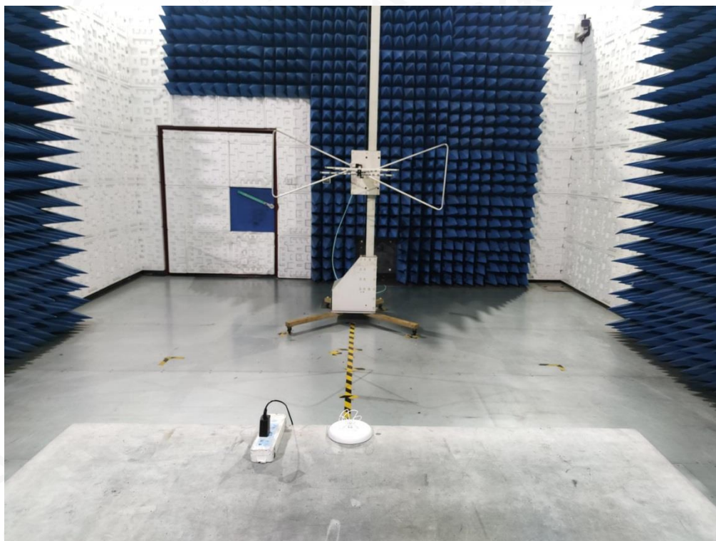
FCC RADIATED EMISSION TEST SETUP ABOVE 1GHZ
