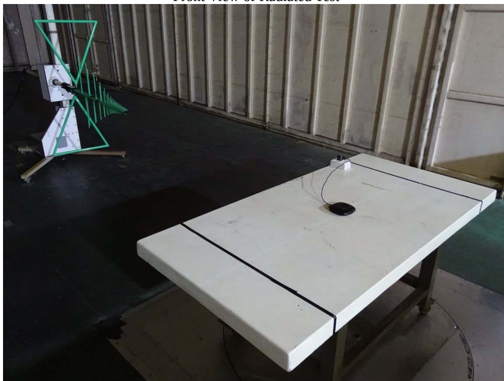
Back View of Radiated Test
