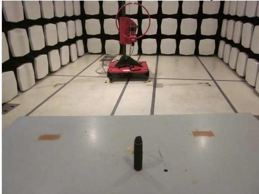
Measurement of Radiated Emission Test Set Up
