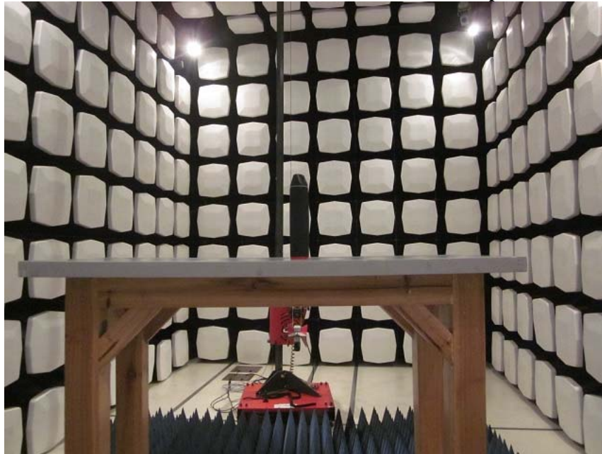
Measurement of Radiated Emission Test Set Up
