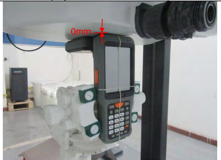
Top Side (Separation distance of 0mm)
