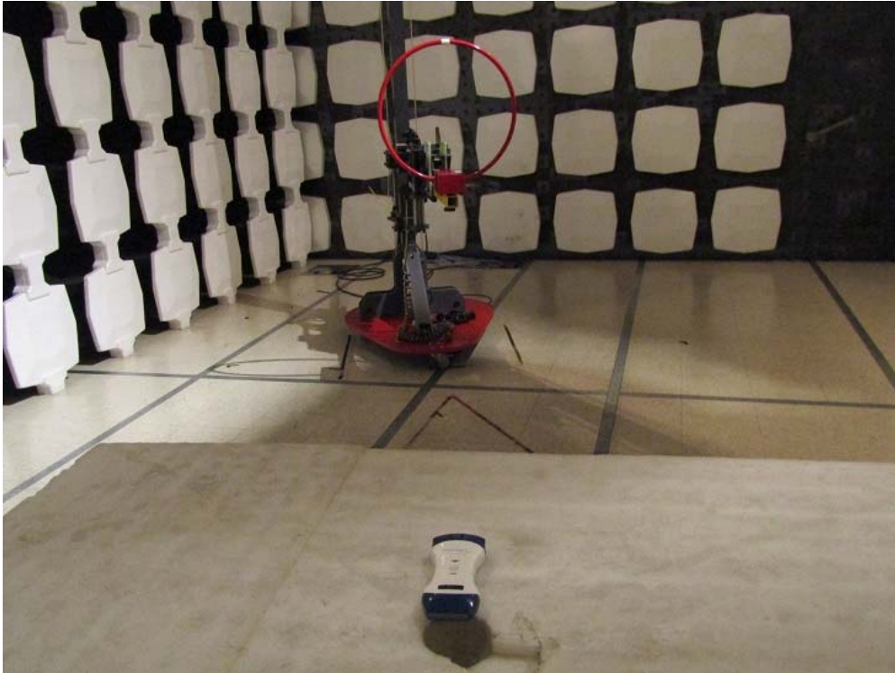
Measurement of Radiated Emission Test Set Up
