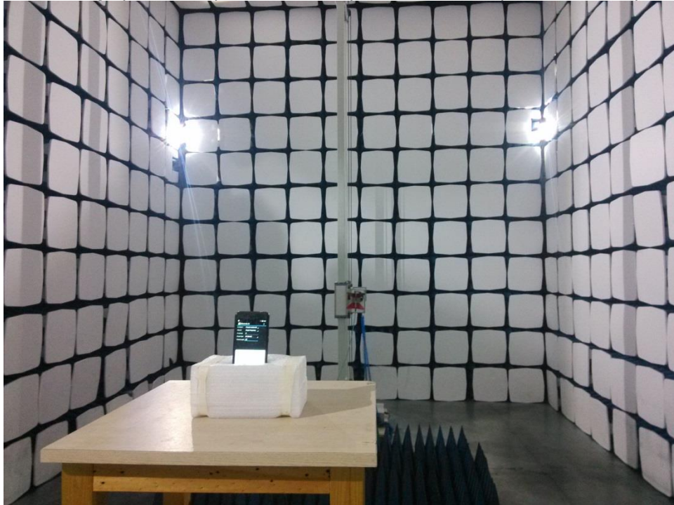
Photograph 4: Set-up for Radiated Spurious Emission above 18GHz
