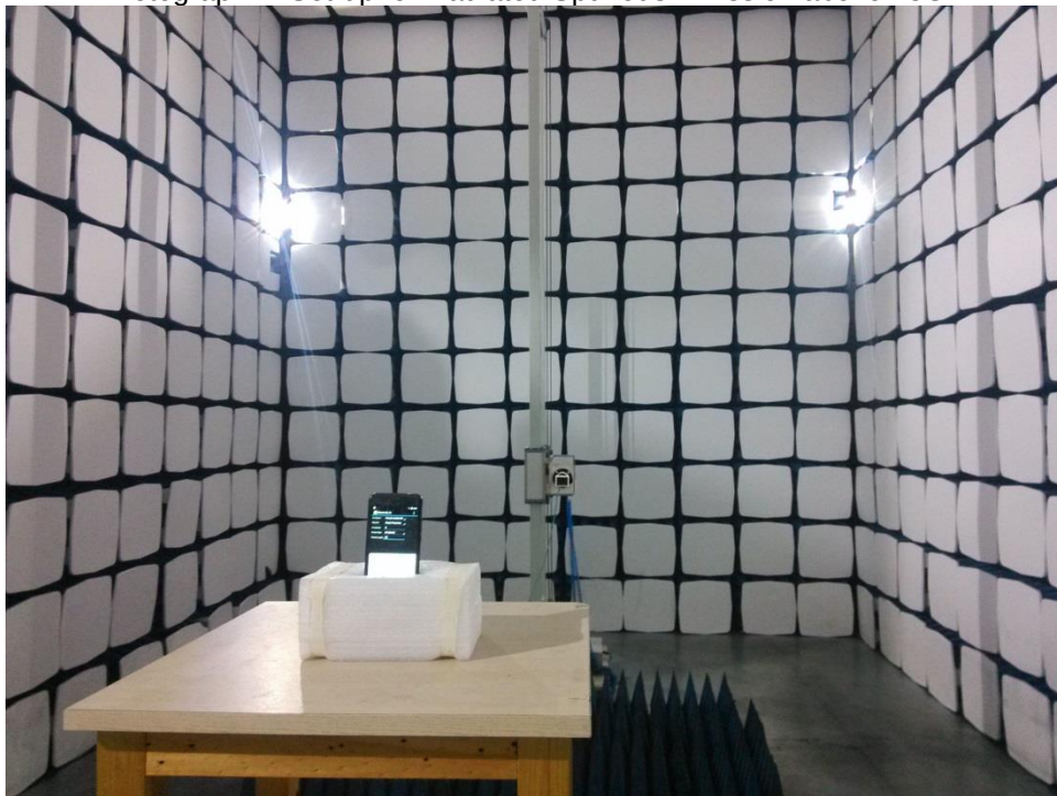
Photograph 4: Set-up for Radiated Spurious Emission above 18GHz
