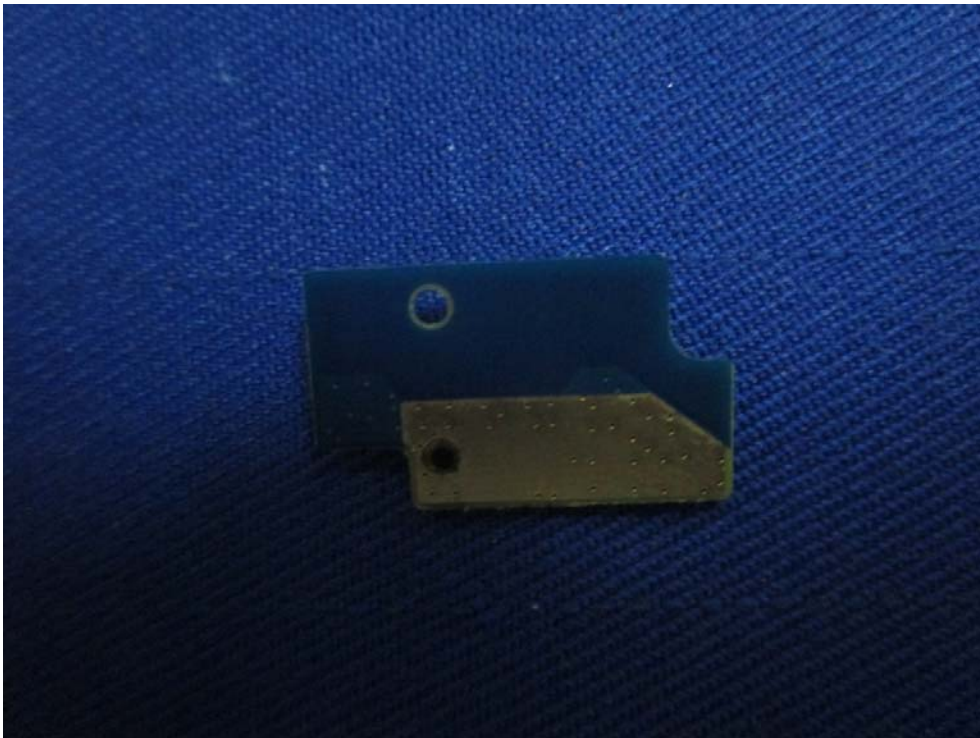
EUT –ANT PCB Back View
