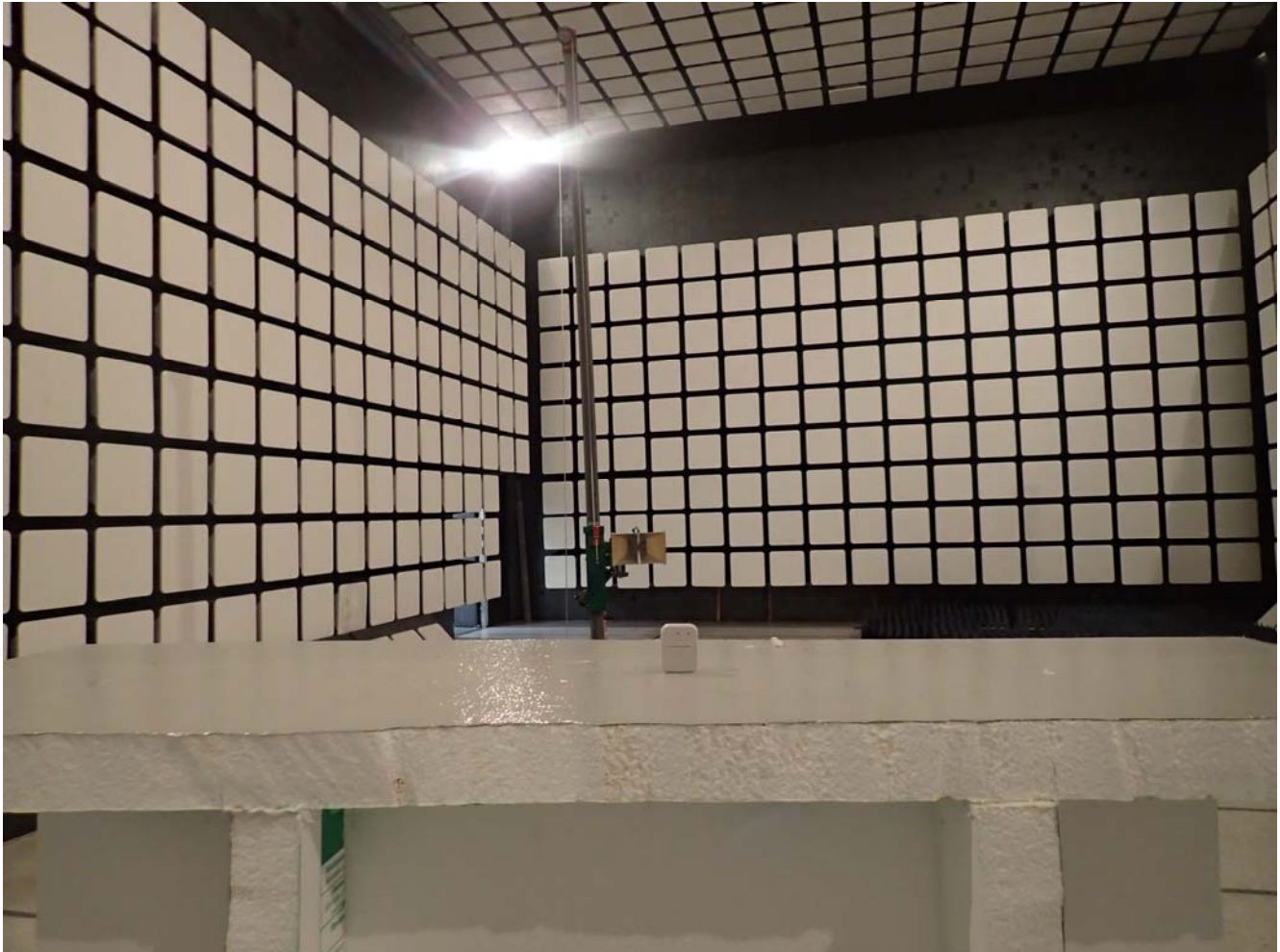
Radiated Emissions @ 3 m Orthogonal Position 3
