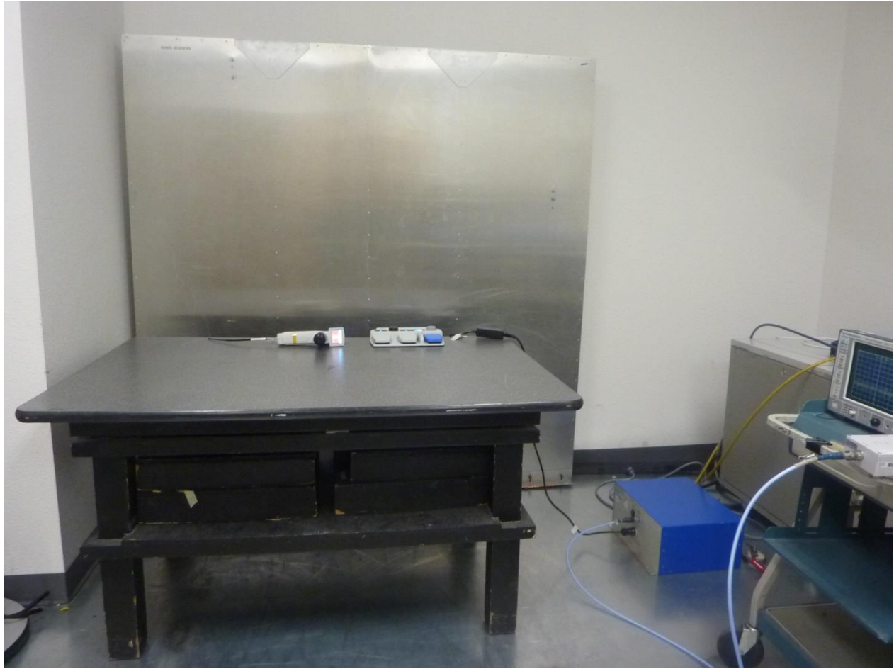
Figure 1: Test Setup for Conducted Emission – Front View
