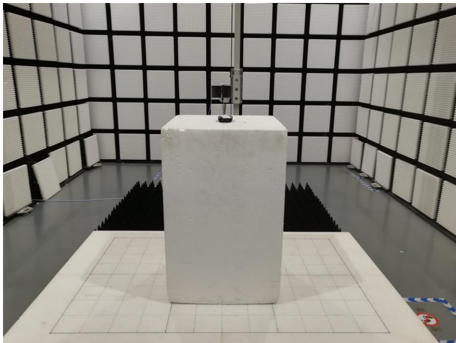
Fig. 3 Radiated emission setup photo(Above 1GHz)
