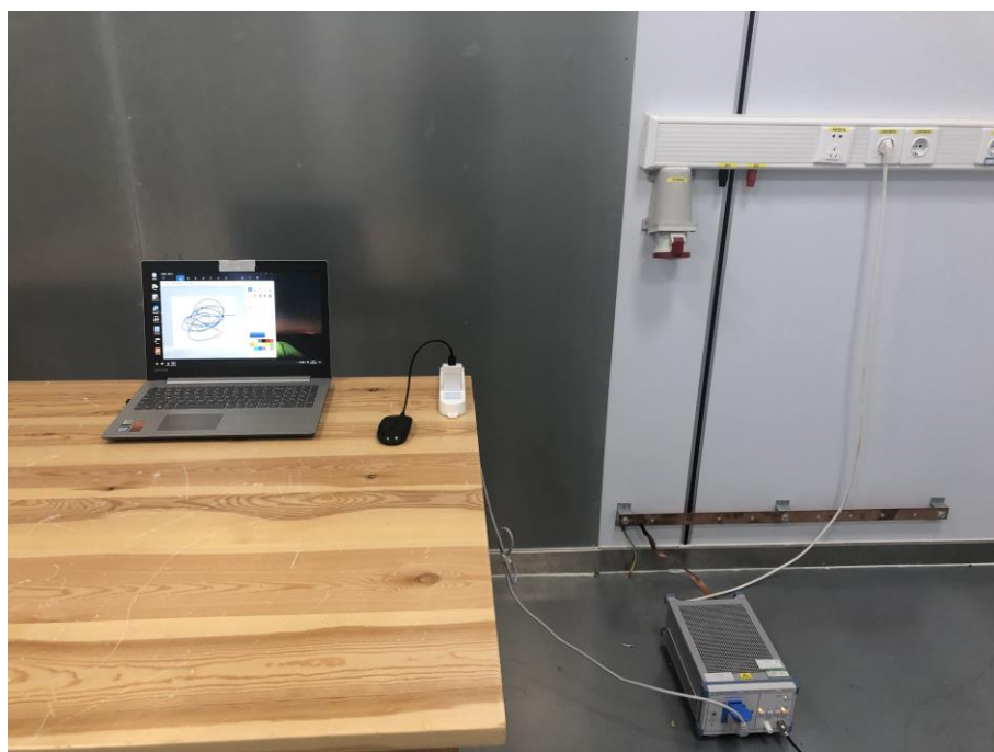
Fig. 4 Power line conducted emission setup photo
