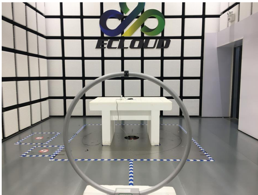
Fig. 1 Radiated emission setup photo(Below 30MHz)
