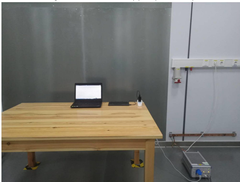
Fig. 4 Power line conducted emission setup photo
