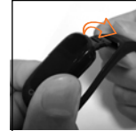
5. Insert the USB charging interface.
