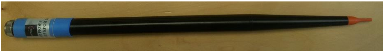
Figure 1 – MVG COMOSAR Dosimetric E field Dipole
